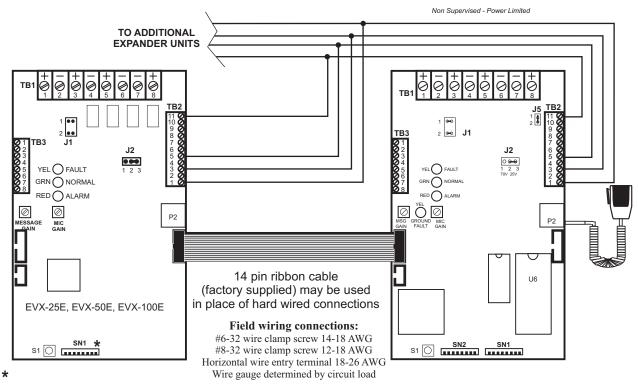
NOTE: Switch SN2-8 must be in the OFF position for all units without Mic attached.
