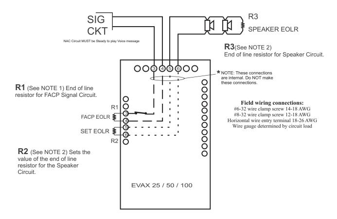
NOTE 1: If the Fire Alarm Signal Circuit requires a 4.7K end-of-line resistor, then R1 must be a 4.7K. Normally, this resistor is connected to the Signal Circuit through a closed Trouble contact. When the EVAX 25/50/100 goes into Trouble, the contact opens, producing an "Open" on that Signal Circuit, notifying the FACP.
